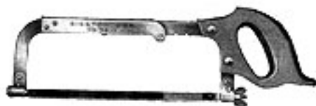
First make certain teeth are pointing away from handle and place holes in blade over both pins.
