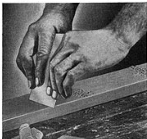
Proper way to hold cabinet scraper
