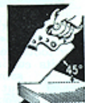
Proper angle for cross-cutting
