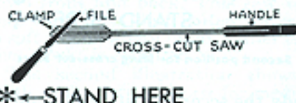
First position for filing hand saws for cross-cutting
