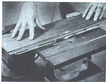
Using same "square board" to cut straight edge on piece of this stock having no straight side.
