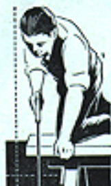
Proper position for cross-cutting
