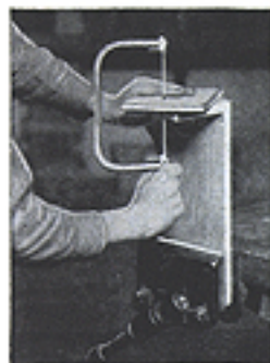
Using coping saw with saddle
