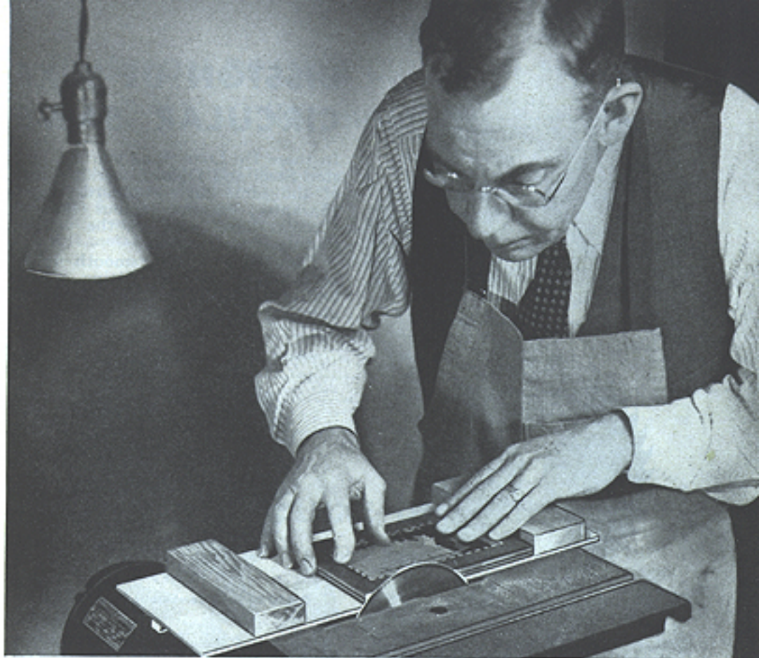
ABOVE—Trimming inlay picture with "square board" made of plywood with a strip to fit table slot tacked to bottom.
