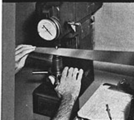
Testing temper after removing saw blade from furnace.
