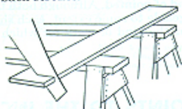
Place board across two sawhorses and cut outside the area they occupy
