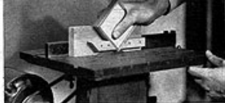
Making cuts for feather-edge joint at corner of small box.
