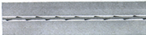
Looking from back of saw, this shows how the teeth, when set, extend beyond the sides of the blade.
