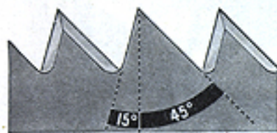
Side view of cross-cut teeth (enlarged)
