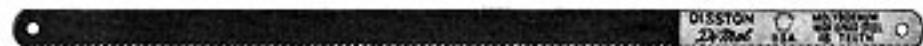
Disston Di-Mol Molybdenum High Speed Steel Hand Blades are made 10 inches; 18, 24, 32 teeth to the inch. 12 inches; 14, 18, 24, 32 teeth to the inch.
